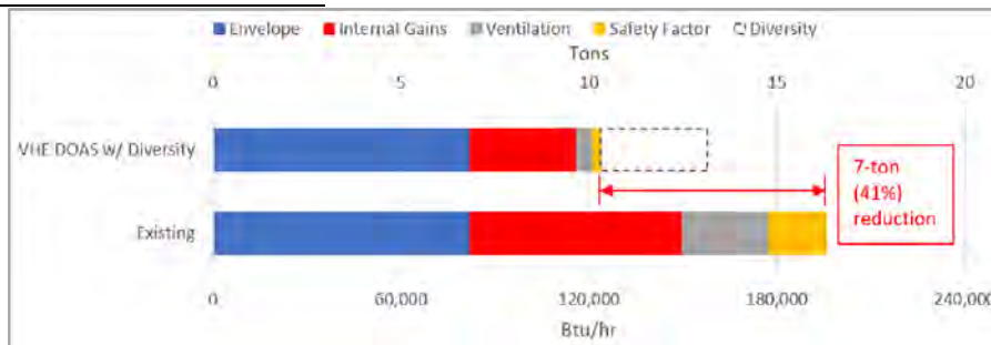
Figure 10. Peak cooling loads from Building #13 resulting in a system downsizing of 41%.
