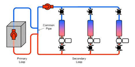
P-S configurations consist of two connected loops—the primary serving the thermal source and the secondary serving the distribution—linked by a common pipe that hydraulically decouples their flows.
