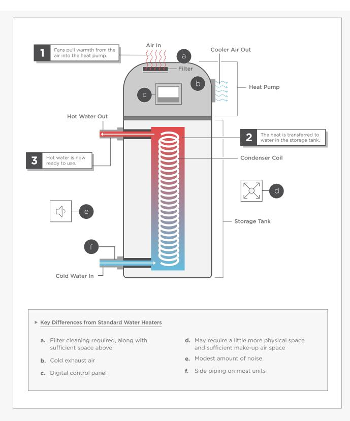
Heat pump waters heaters have several unique installation requirements in comparison to standard electric or gas water heaters.
