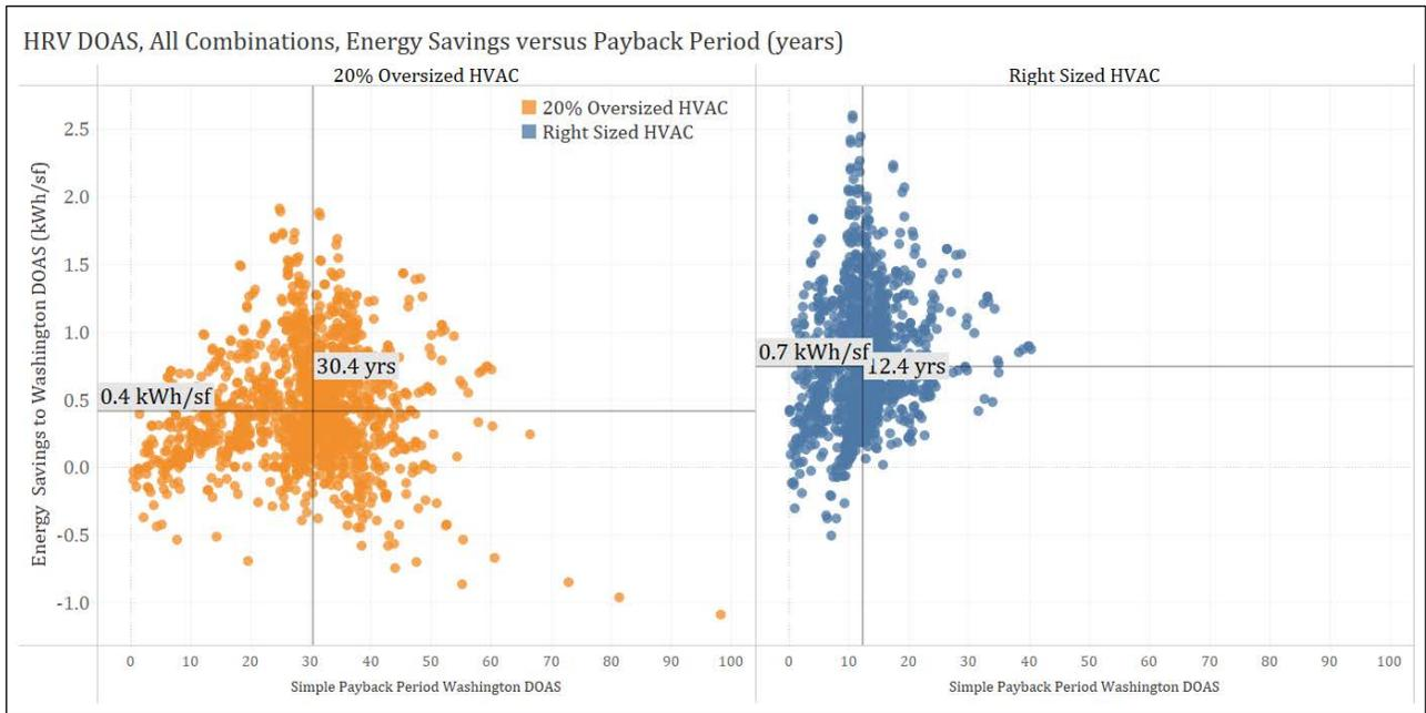
**Figure 6: HVAC energy savings of each configuration versus the Washington 2018 energy code DOAS configuration by the payback period of the system in years. Information highlighted based on how cooling and heating systems are sized.**
