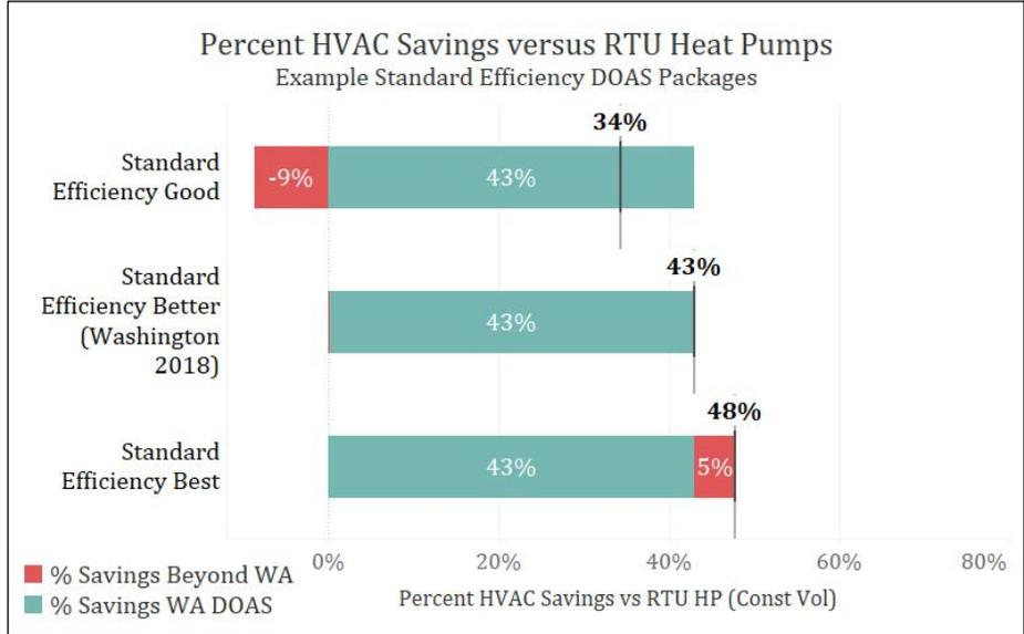
**Figure 19: Percent HVAC savings versus RTU Heat Pumps for Standard Efficiency DOAS packages**
