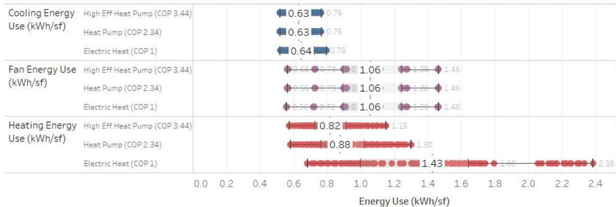
Post heating coil efficiency parameter, individual results of energy analysis averaged by end-use.
