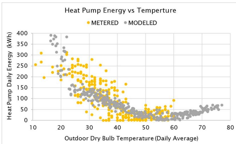
The modeled performance curves are typically based on current test and rating procedures that do not take into account actual system behaviors in certain ambient conditions. System COPs are assumed to vary directly with the difference between outdoor ambient temperature and indoor temperature, with compressor capacity and efficiency declining smoothly as outdoor ambient temperature declines.
