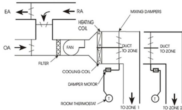
Because the air must be tempered, ventilation air is introduced as part of the supply-air stream that is divided between the two coils. This ventilated air is not based on occupancy in a zone, as zoning is based on heating and cooling loads. All in all, this is a very inefficient way to heat and cool a building.
