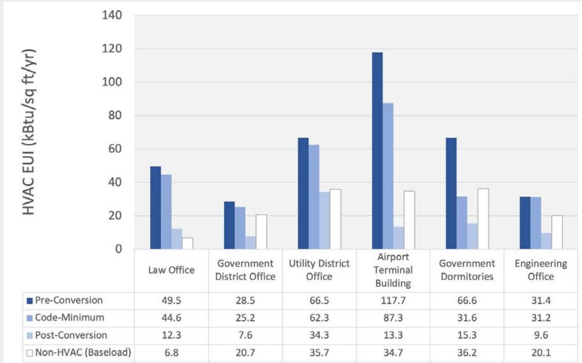
The large code minimum savings in the airport terminal building are due to the elimination of the very inefficient existing dual-deck RTU systems that resulted in a significant amount of simultaneous heating and cooling during many hours of the year. In the government dormitory project, the large code-minimum savings come from the elimination of the existing electric-resistance heating in the starting actual case, substituting minimum efficiency heat pump systems for the code-minimum case.
