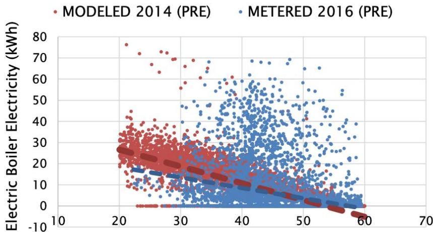
The modeled range (red) produces a tighter hourly pattern than that exhibited by the metered data. Additionally, there are many more metered readings well above the curve, especially in the 40–50 F ambient conditions. Another example looks like this:
