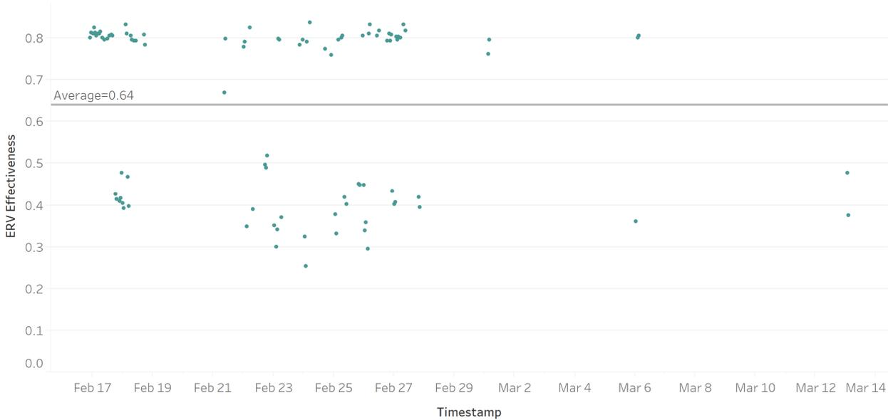
FIGURE 21: UNIT B (BOLT-ON ERV) AVERAGE HOURLY EFFECTIVENESS (UNFILTERED)
