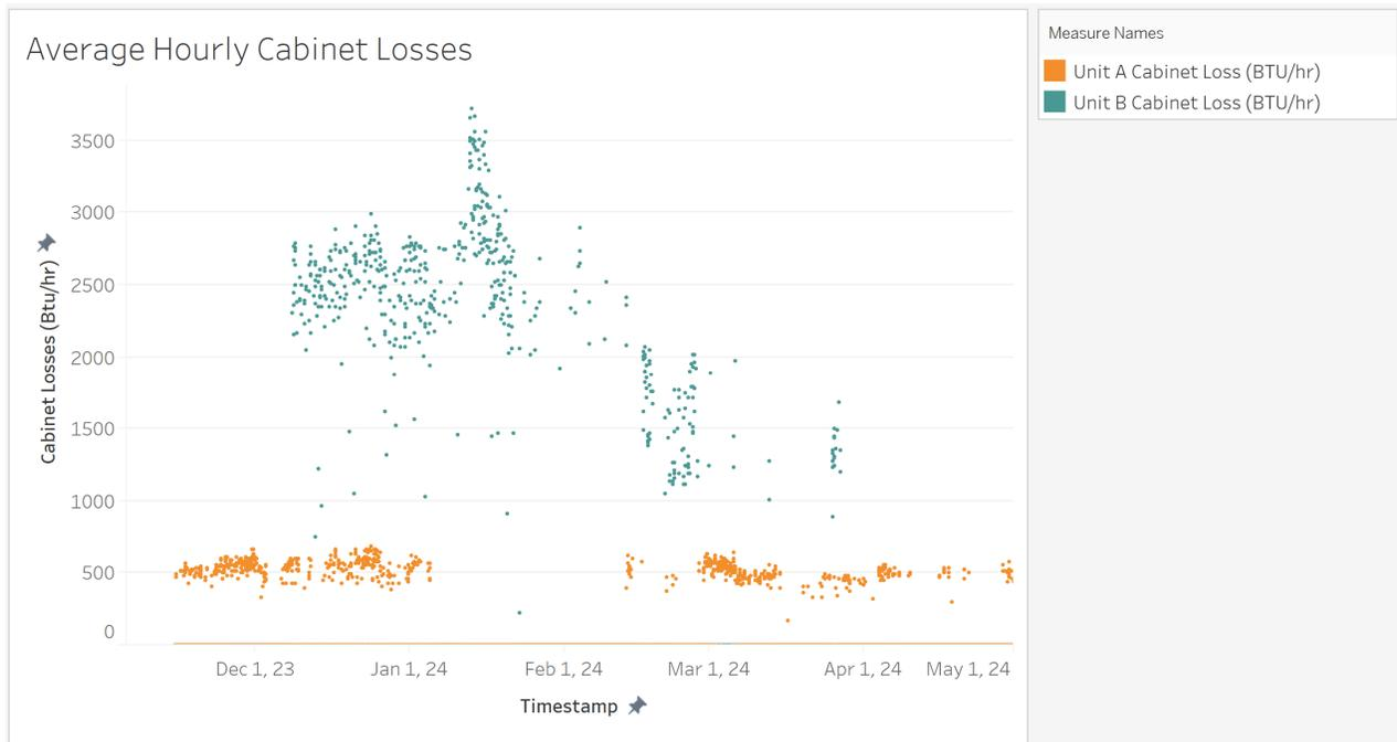
FIGURE 28: AVERAGE HOURLY CABINET LOSSES IN UNITS A AND B
