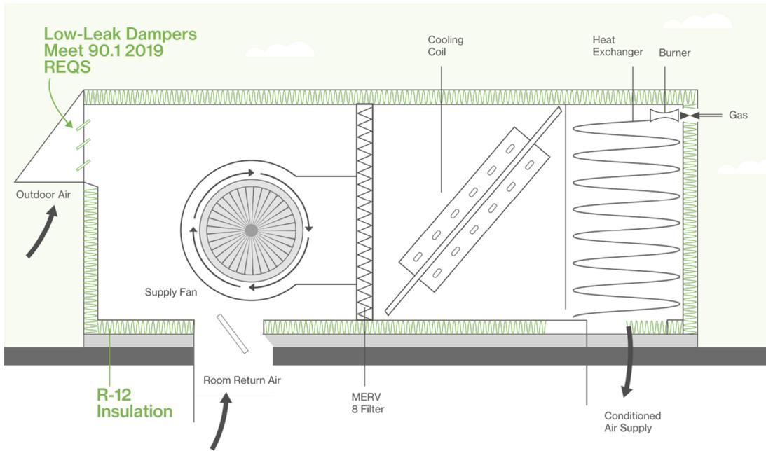
FIGURE 3: TIER 1 ERTU SCHEMATIC DIAGRAM<sup>4</sup>
