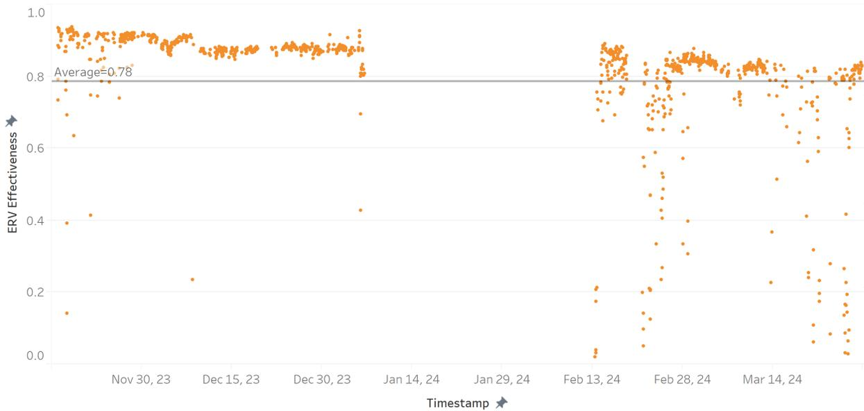
FIGURE 20: UNIT A (INTEGRATED ERV) AVERAGE HOURLY EFFECTIVENESS (UNFILTERED)
