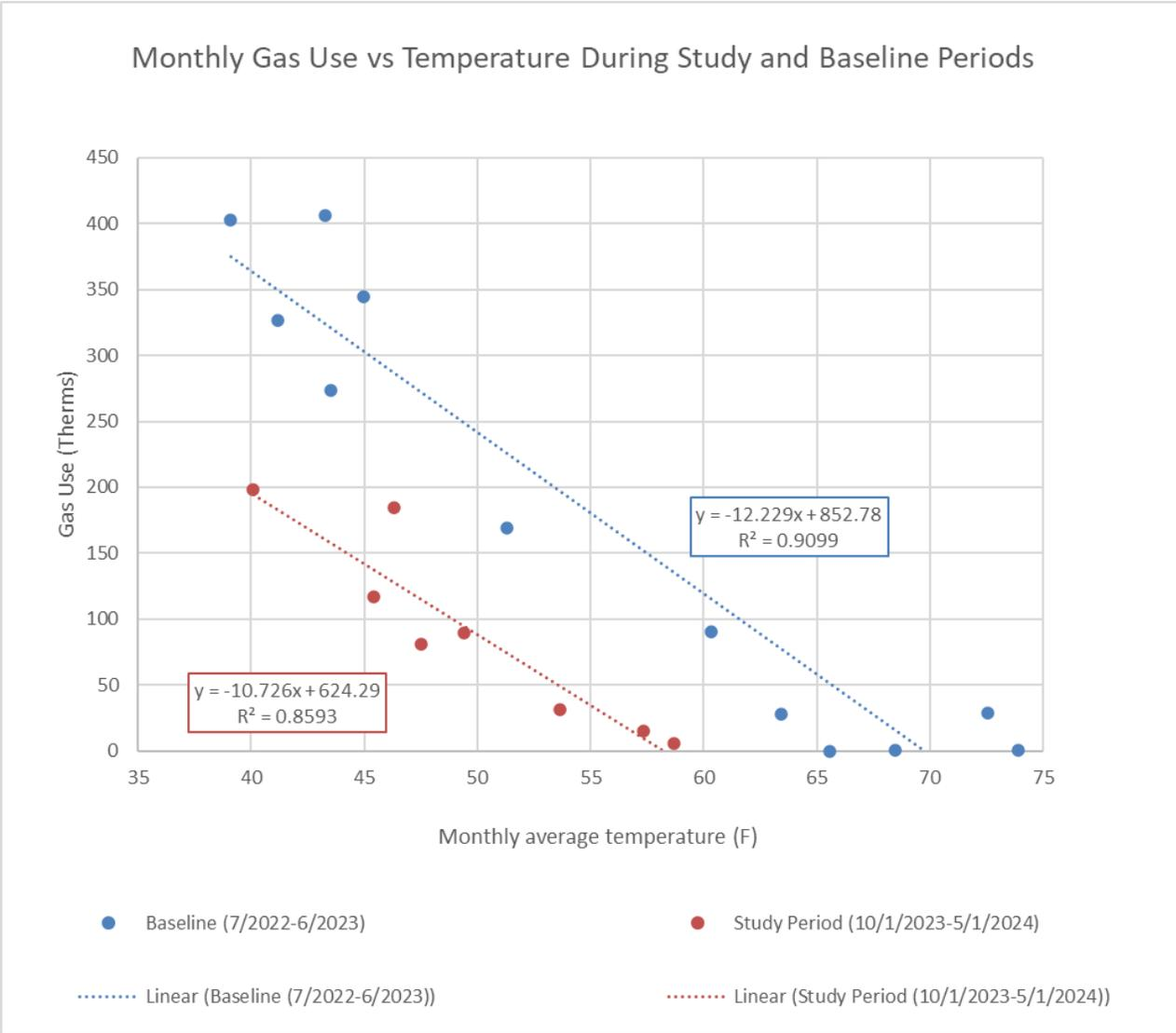
FIGURE 17: MONTHLY GAS USE COMPARED TO AVERAGE MONTHLY TEMPERATURE IN THE BASELINE AND STUDY PERIODS
