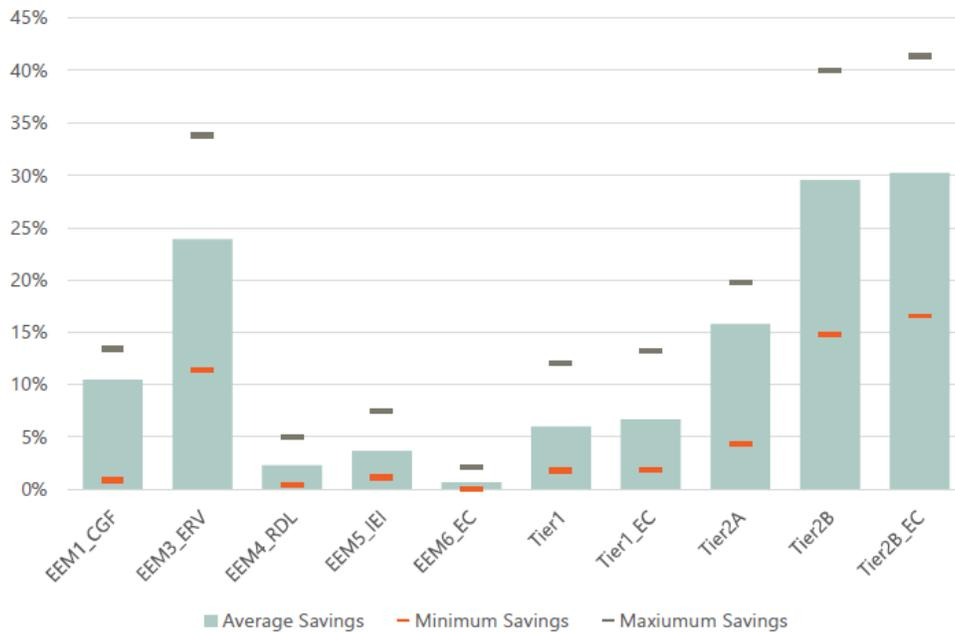
FIGURE 7: AVERAGE, MINIMUM, AND MAXIMUM HVAC EUI SAVINGS ACROSS BUILDING TYPES AND CLIMATE ZONE FROM CADEO REPORT
