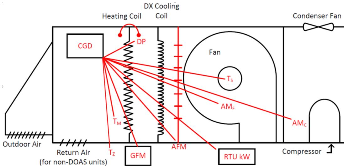
FIGURE 13: RTU METERING SCHEMATIC
