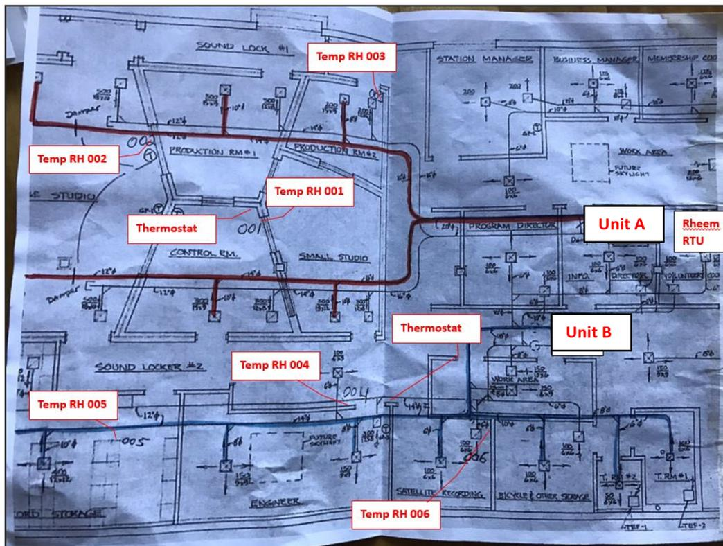
FIGURE 14: ZONE AIR TEMPERATURE SENSOR LAYOUT
