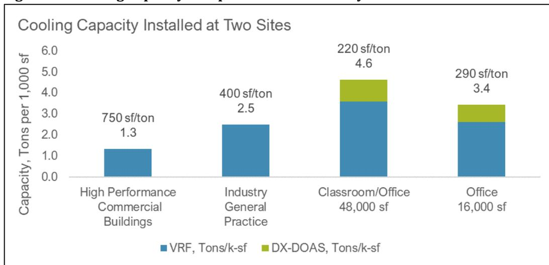
While the cooling capacity of the space conditioning system could have been reduced when accounting for ventilation air being delivered at colder temperatures, 60 °F or 65 °F, compared to a typical building's setpoint (75 °F), these sites' total installed tonnage suggests that most DX-DOAS designs with VRF do not account for this capacity or the DX-DOAS units fully reheat the air to a neutral temperature of 70 °F or higher.
