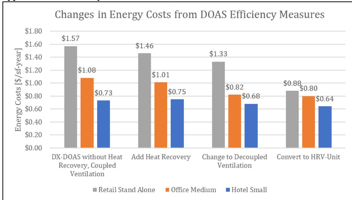
The review of energy analysis from applying incremental changes in the DOAS configuration shows the greatest reductions in energy costs by decoupling the ventilation air in the small hotel and medium office, and by converting to an ERV/HRV unit in the stand-alone retail building. The small hotel shows a minor increase in building energy costs when adding heat recovery to a DX-DOAS unit in this climate zone.
