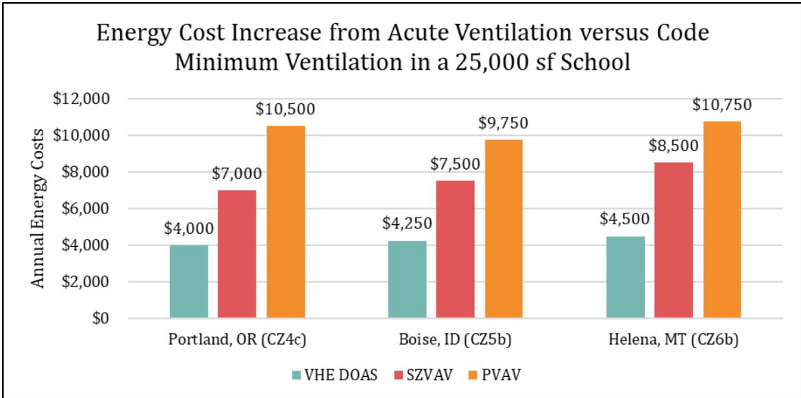
**Figure 2: Operational energy cost increases per year for a sample small school under acute ventilation operations vs code minimum ventilation operations. Simulated results for three climate zones, CZ4c, 5b, 6b.**
