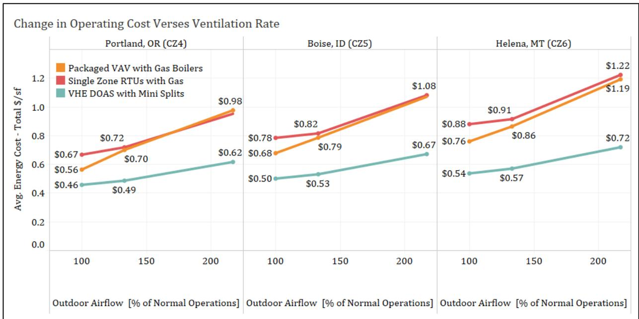
**Figure 4: Operational energy cost results from the energy analysis for each system versus the percent of operational outdoor air for new buildings in climate zones 4c, 5b, 6b.**
