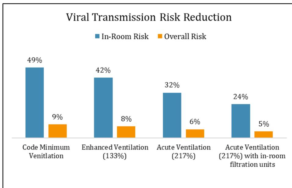
**Figure 1: Viral Risk Reduction: Increasing Mechanical Ventilation Rates in the 5-Classroom Scenario.**
