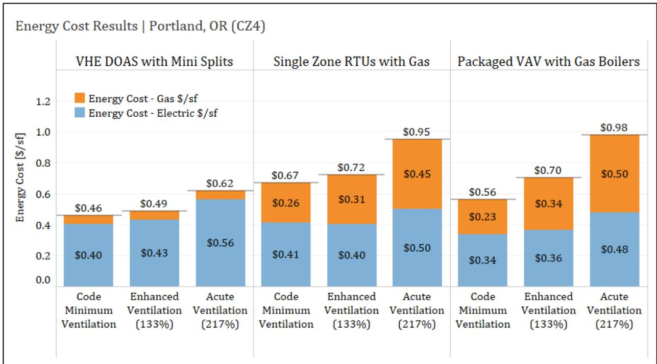
**Figure 3: Whole building energy modeling results of operating costs under normal, enhanced, and acute operations. New buildings, Portland, OR.**
