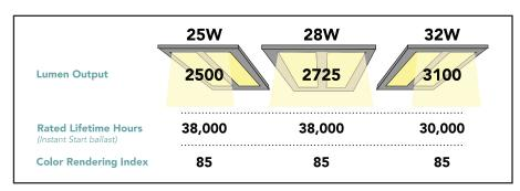
\*Numbers taken from Philips models: 25W F32T8/ADV835/XEW/ALTO • 28W F32T8/ADV835/EW/ALTO • 32W F32T8/ADV835/ALTO
