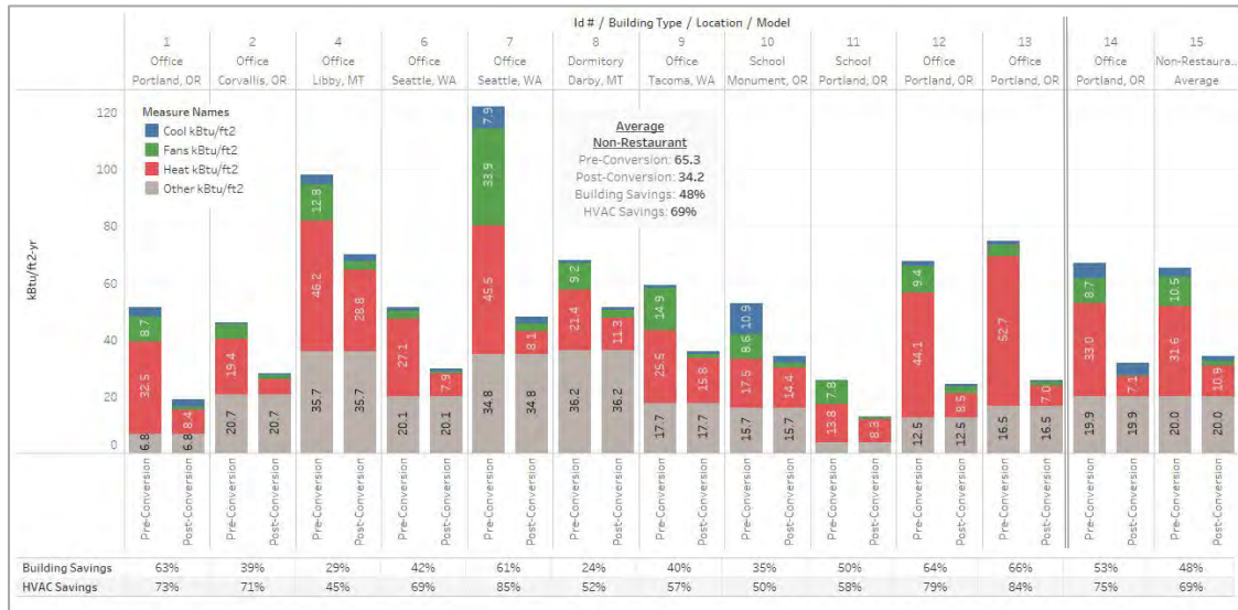
Figure 4. Annual energy use intensity by end-use pre- and post-conversion. Average non-restaurant project savings are 48% of total building energy use and 69% of HVAC energy use.
