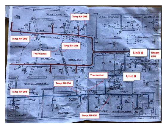
FIGURE 14: ZONE AIR TEMPERATURE SENSOR LAYOUT
