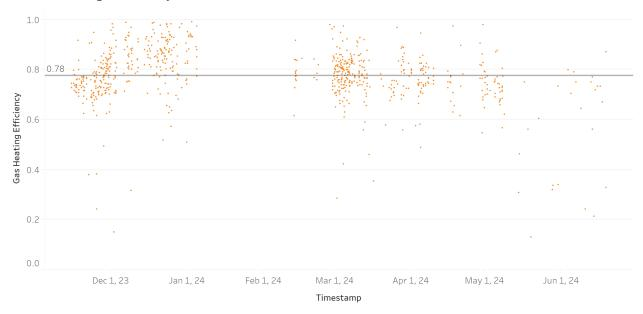
FIGURE 18: UNIT A AVERAGE HOURLY HEATING EFFICIENCY
