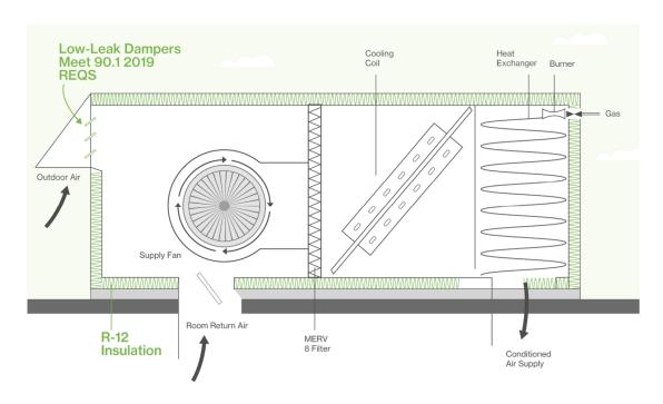
FIGURE 3: TIER 1 ERTU SCHEMATIC DIAGRAM<sup>4</sup>
