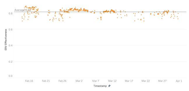
FIGURE 22: UNIT A (INTEGRATED ERV) AVERAGE HOURLY EFFECTIVENESS (FILTERED OUT <70%)
