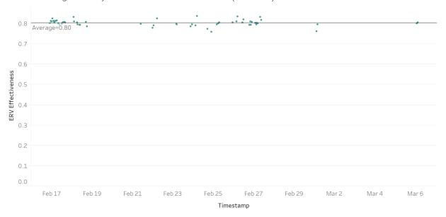
FIGURE 23: UNIT B (BOLT-ON ERV) AVERAGE HOURLY EFFECTIVENESS (FILTERED OUT <70%)
