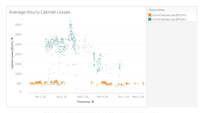
FIGURE 28: AVERAGE HOURLY CABINET LOSSES IN UNITS A AND B
