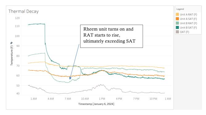
FIGURE 29: THERMAL DECAY OF SUPPLY AND RETURN AIR TEMPERATURES IN BOTH UNITS
