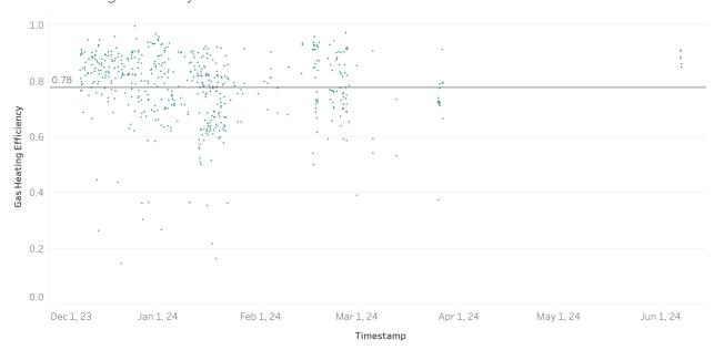
FIGURE 19: UNIT B AVERAGE HOURLY HEATING EFFICIENCY
