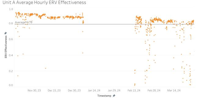
FIGURE 20: UNIT A (INTEGRATED ERV) AVERAGE HOURLY EFFECTIVENESS (UNFILTERED)
