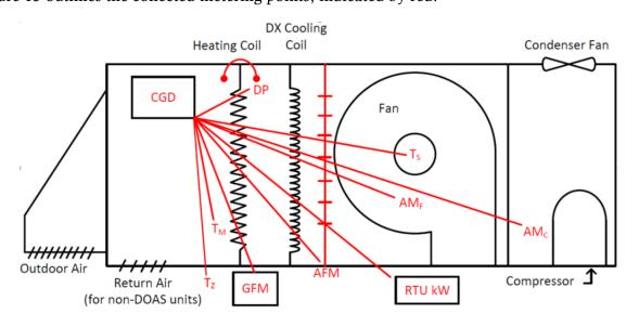
FIGURE 13: RTU METERING SCHEMATIC
