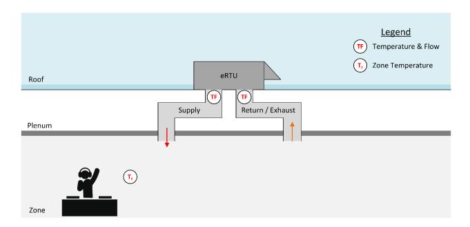
FIGURE 15: ZONE, SUPPLY, AND RETURN TEMPERATURE METERING SCHEMATIC
